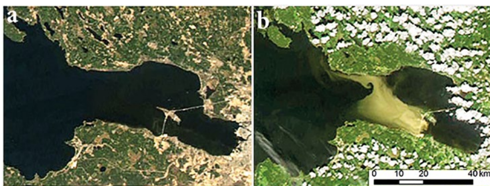
Figure 22. Impact of the works related to the construction of Bronka: a view over the area. A: before hydro-technical works started (20 th April, 2014), B: at the time of hydro-technical works (7 th July, 2014). Source: Sukhacheva and Orlova (2014).
