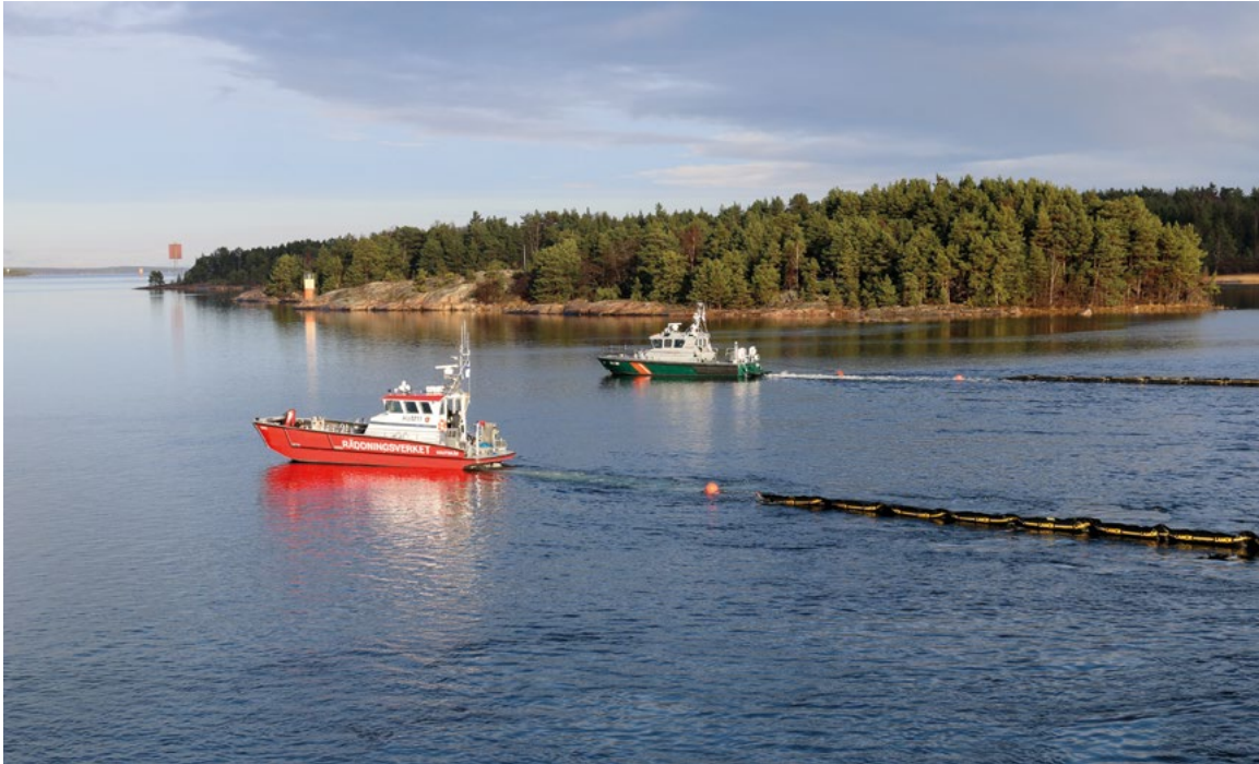
For once, the weather is nice in November. The boats of the Finnish Border Guard and the Southwest Finland Emergency Services together pull an oil boom in the Archipelago Sea. Photo: Jouko Pirttijärvi.
