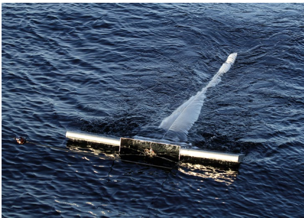
Figure 4. A Manta trawl in action. Manta is a special type of a surface neuston net with a mesh size of 0.33 mm. It is presently used globally for collecting surface microlitter. Photo: Mika Raateoja.
